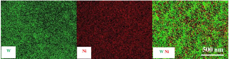
Fig. 9. EDS mapping of the combustion product (W-Ni) after SPS consolidation
