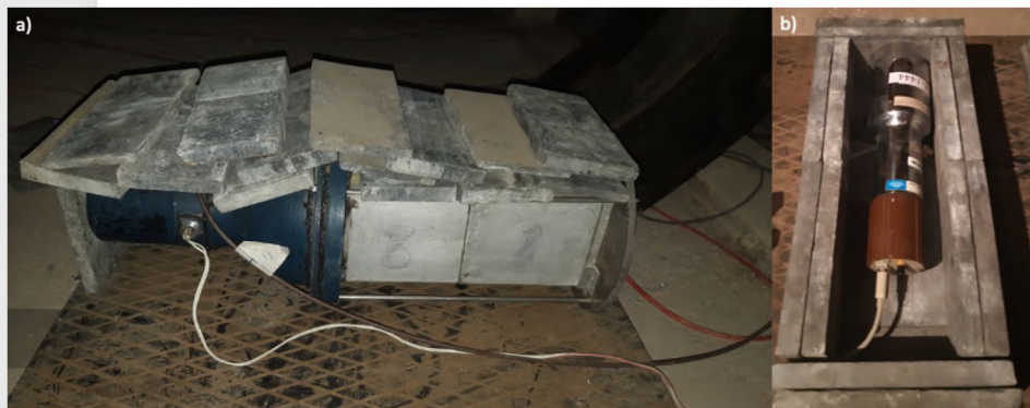
Figure 1. Large NaI spectrometer with lead filters above a); ORTEC spectrometers with lead filters from the sides and the bottom b).
