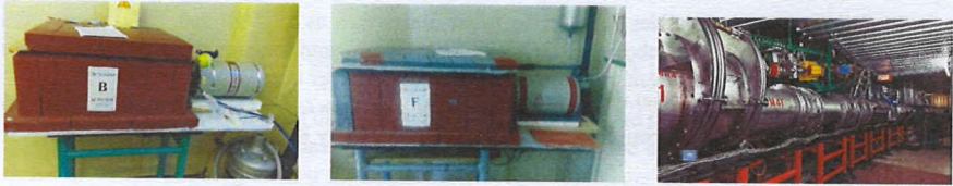
Figure 1: Left and center: HPGe detector setup used for off-line \gamma -ray measurements. Right: General view of the Nuclotron accelerator at VBLHEP, JINR, Dubna.
