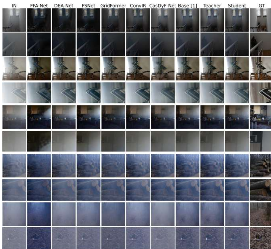
Figure 10: Qualitative dehazing comparison on O-Haze, I-Haze, and Haze4K for the KD framework. Teacher and Student closely match in visual quality while achieving over 150\times speedup.
